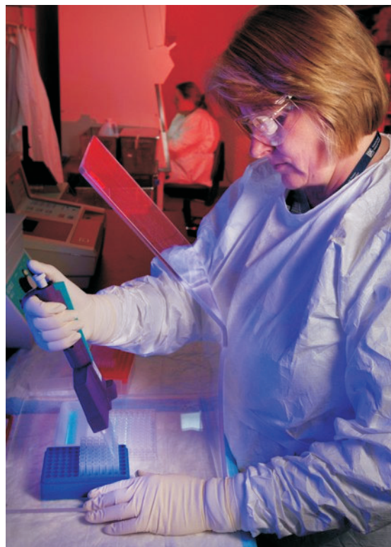
FIGURE 3. A micropipette with multiple tips allows for more rapid ELISA tests. (Courtesy, CDC)
