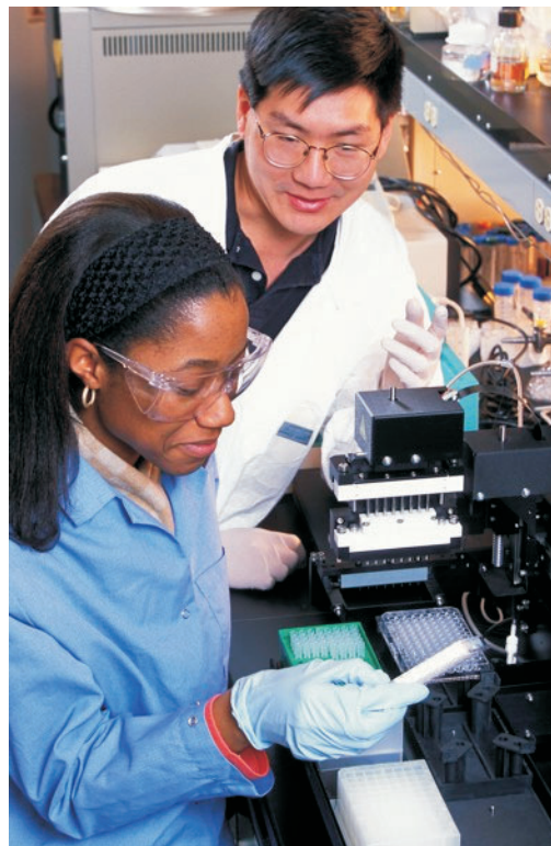
FIGURE 1. These lab technicians are wearing PPE consisting of lab coats, gloves, and eye protection. (Courtesy, Agricultural Research Service, USDA)
