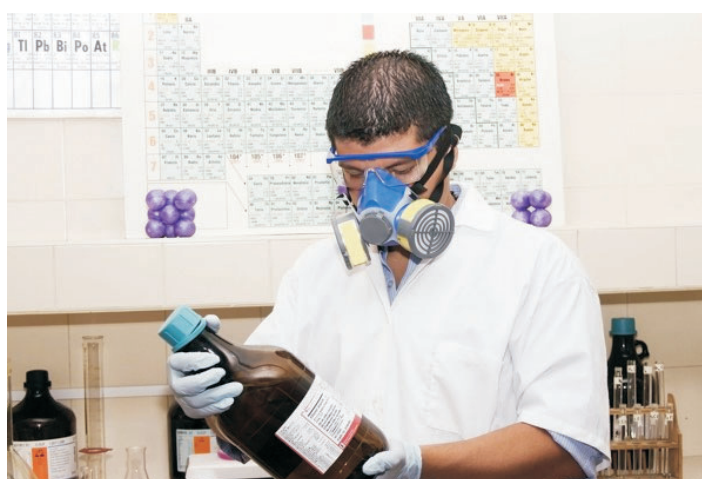
FIGURE 3. A chemical cartridge respirator provides protection from fumes, vapors, and other gases.
